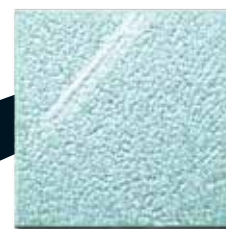
Breaking pattern of tempered safety glass
