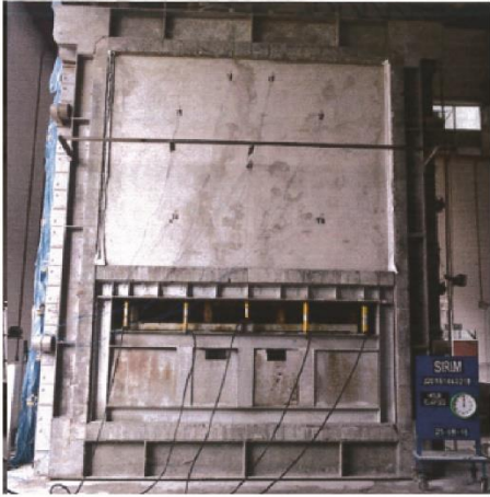
The exposed face of the wall system before the test
